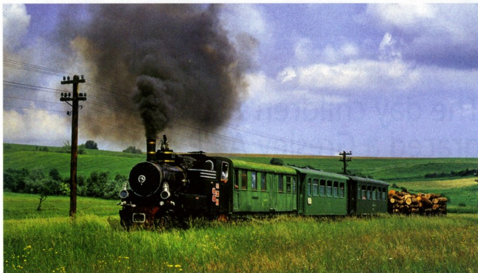
Romanian steam: On June 8, 1995, No 764-155 heads a train away from Agnita on the 2ft 6in gauge line to Sibiu. The train is a tourist special, but the opportunity has been taken to add some freight wagons, carrying timber, behind the three carriages. Built at the delightfully named August 23 works in Bucharest in 1949 (works number 521), the 0-8-0T was withdrawn in 1997 and stored at the narrow gauge depot in Sibiu, but with two other steam locos has recently been unexpectedly moved to another site. JIM BALLANTYNE
